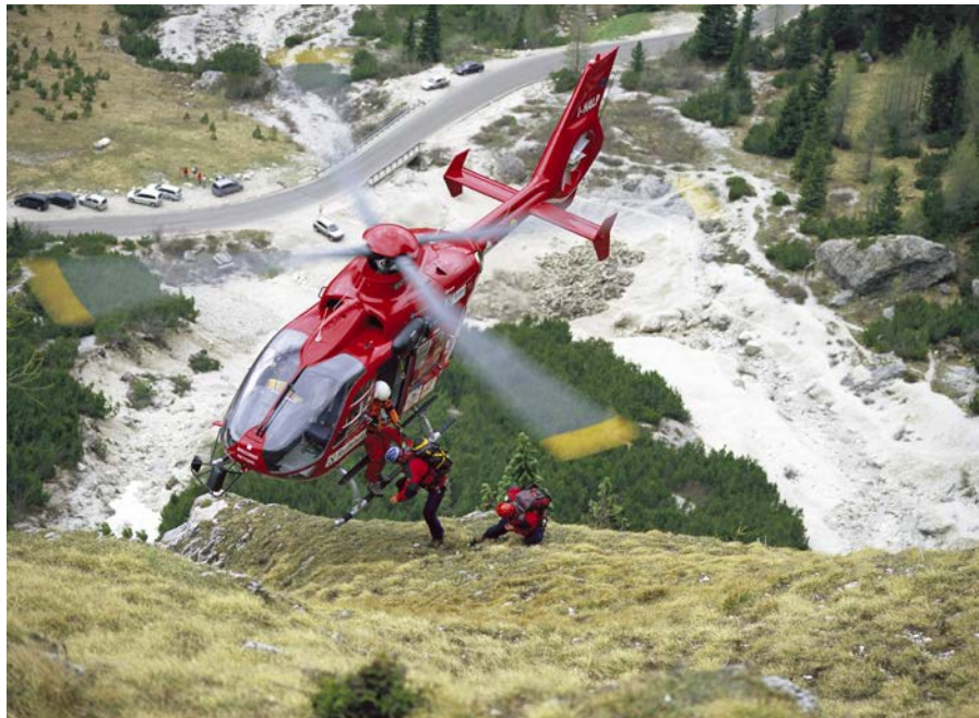
Figure 15- Toe-In Landing. Using a Eurocopter EC 135 T2, rescuers from the Italian rescue association Aiut Alpin Dolomites, conduct a toe-in landing near the Passo Sella in the Dolomites. Image copyright Mateo Taibon.
