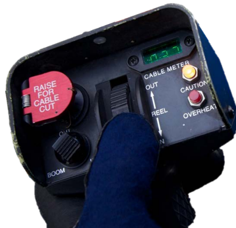
Figure 26- Cable cutter control. Red guarded switch on hoist pennant control. Image courtesy Travis County STAR Flight, Texas.
