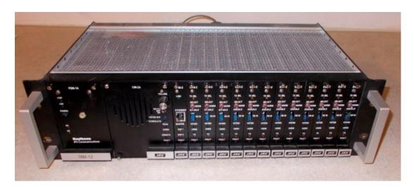
• PSM, being the power supply module. It inputs either the 110v AC or 12v DC to convert a +12v and -12v-rail voltage for all the other modules.
