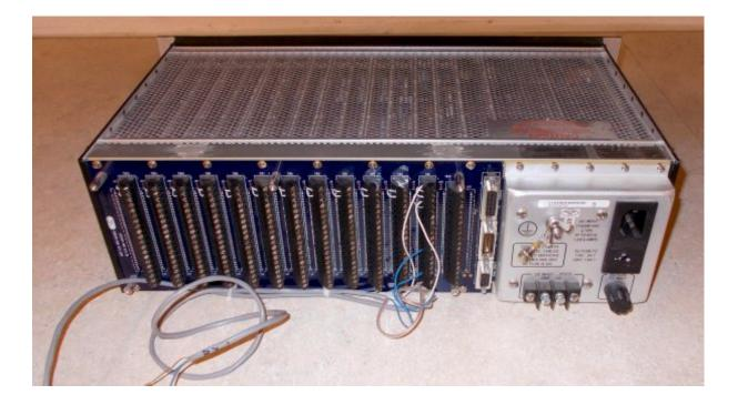
Shown here is the unit in service at the MCP. Most of the SVM connections were made with wires following the resistor color code for easy tracing. Shown above the SNV-12 is an audio switcher (TDV) to facilitate a flat audio system to which the SNV-12 won't accommodate.
