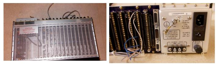
Showing below is the rear during bench testing. A handy ground pin jack as been added on both the front and rear for measurements.
