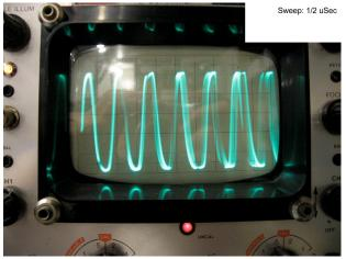
The image shown here is a normal, clean tone observed on an oscilloscope during alignment (3 KHz deviation into a receiver).
