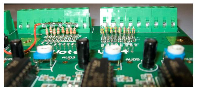
If you note carefully you'll see that some of the resistors are mixed values. This picture was taken during R&D experimenting with different values for both COR and audio inputs.
