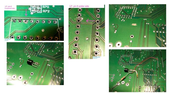
Then a ground spot was created (for the transistor) by scraping away a block of the (green) PCB covering to expose the copper ground. It was tinned and the transistor's emitter lead was soldered there. The resistors and jumper wire were added with shrink, where appropriate. Parts used were a 2N3904, a tiny wire jumper and two 10K resistors, one being 1/8 watt for appropriate close area consideration.
