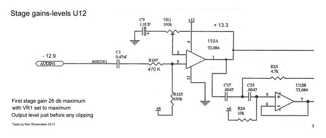
Note: In the event your receiver's TLP is lower than -13 leave the input resistors (R107~R114) as OEM.
