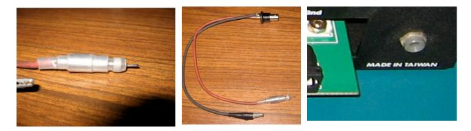
During alignment you are asked to adjust the pots while probing test points. The "Noise-x" TPs and pots are properly spaced apart for easy test pin insertion and pot adjustment as shown in the left image. However, the "AUD-x" TPs are in a tight area as seen in the right image. Performing the above modifications to your probe avoids slippage and possible damage to a circuit.
