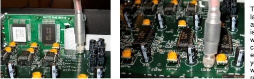
The second to the last step in the alignment procedure is assuming you wish the voter's channels weighted evenly. In the case you have a problem with an input receiver being
