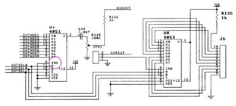
There's another circuit similar to U7 and its function. Looking at U8, being an 8channel indication (or control) output, for external equipment does address pin 6 to some degree. With JPR1 in the "1" position enables the output all the time therefore, the indication would stay
