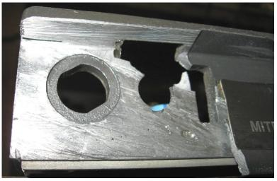
The last area to cut is on the inside where the key parts where located. Make the cut for this as well.
