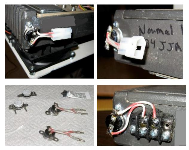
Shown on the left is the compound used to transfer the heat to the switches.
