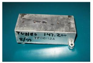
For final tuning this filter needs to be in the OEM circuit arraignment (driving the PA) and observing the RF level at transmitter output port.
