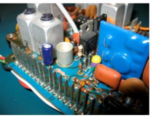
Here's the modified exciter board to the extent wires are soldered to the P902 (I/O) pins with heat shrink to increase reliability. Some of the unused pins are removed to assist the ferrite bead clearance (some others are left). The beads can reduce RFI on the lines if the site is (RF) hostile.
