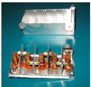
Z501 comes in two band ranges. Model TFD6111 is the (L) 132~150.8Mhz range and the TFD6112 is the (M,H) 150.8~174 range. As shown above, the "L " range won't need any tuning or modifications for the 144~148 MHz amateur radio band (2-meters).
