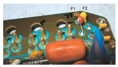
Shown on the left are the two audio coupling capacitors that now use the (old) F4 line as the input (flat audio). TLP is about +3.2 dbm.
