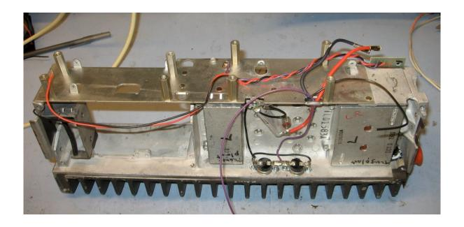
The picture above is before the exciter is installed. Did you notice the two silver "boxes"? They are filters for the transmitter. The one on the left is a band pass filter (Z501) for the exciter board's output.
