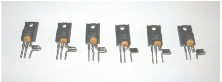
Shown are several units being made as a production "line" to produce several transmitters with their regulators.
