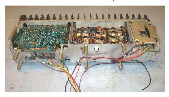
Now, you can install the exciter board in the chassis as show here. Then install the wiring for the power control board; 3 wires; ground, A+ and control voltage. The latter connects to the PA control transistor. In this view a feed-though cap was used however, OEM just has the wire go through a hole in the chassis.
