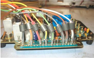
A drop of glue will keep them in place. The unused pins that were removed are 2,3,5,6,10 and 14.
