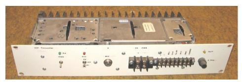
Serial 2 changed to the white panel standard. Shown here is the front of a finished transmitter. Notice there's a switch function to "lock on" the PTT line for transmitter testing under load. It was decided a ON-Center OFF-ON switch is sometimes awkward to use; disable being in the "center" position; one may run the switch to the down position and keep the PTT on, so this was changed to a ON-ON switch as shown below.
