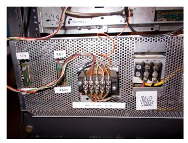
The Author removed the soldered power leads. With spade lug and a terminal block it provides easy troubleshooting in the event a chassis has a problem, such as a short. Plus it's a good point to add an accessory such as a fan or ID unit, etc.
