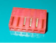
A problem found was intermittent power out. It was trouble shot to a badly corroded plug (and jack) on the interconnect board. P1004. Only three points are used, the A+, A- and control voltage.
