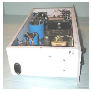
Shown is the rear and the side vent for the fan which is controlled by thermostats mounted on the heat sink of the diode rectifier of the 10-volt supply section. Yes, the Author drilled all those little holes by hand drill. Now, it will be different with version 2.
