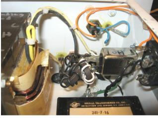
Then the line wires are looped through a set of toroid rings for FM-broadcast sites. The number of turns were determined by sweeping the area of 88~107 MHz. As shown on the right image.
