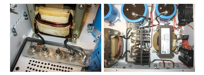
This is the other side of the rectifier. The heat sinking is done directly to the chassis. As previously mentioned, special type of reverse set of diodes are used so the anode goes to chassis ground. The common ground point is shown on the lower left image. On the right is the 10v fuse array. Version 2 with have an ATC fuse external on the DC (red) line cord.
