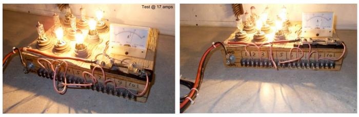
To measure currents greater than 30 amps (as the fixture is set for) the Author built and calibrated a shunt device to work with the Fluke 77 meter, as a 10:1 converter. Therefore, 1 amp on the meter = 10 amps on the test circuit, etc. The Author used automotive headlights (in parallel) to provide a safe, effective load for this test.
