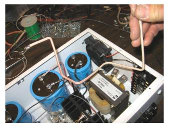
Being assembled here is the ripple filter section for the 10-volt section, with a 1mh/30-amp choke in the center. This was the most expensive part of the whole project.
