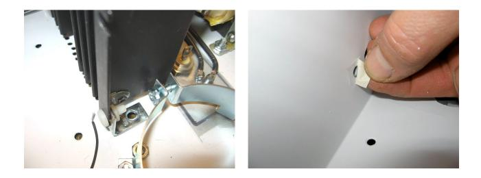
There's twenty on the bottom, less the airflow holes, which, again will depend on the density you choose for them. For the ground connections you'll need to mask off so the painting keeps it clean. This is for the heat sinking for the diodes and a few ground connections. For the latter, you might hit them with a wire brush to ensure a good electrical connection. This can be done before or after painting. For version 2 the hole count may be different.
