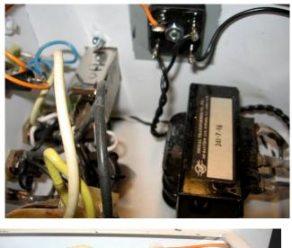
This is the AC entry area and the 12-v section. T2 was easy to find, by "Signal Transformer". The picture below is another view of the 12v transformer, plus shows the AC entry IEC (RFI filter) point. Some surge protection was used. with some MOVs on the AC input.
