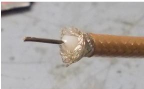
braid a little. This will facilitate it clearing the connector when it's slid on.
